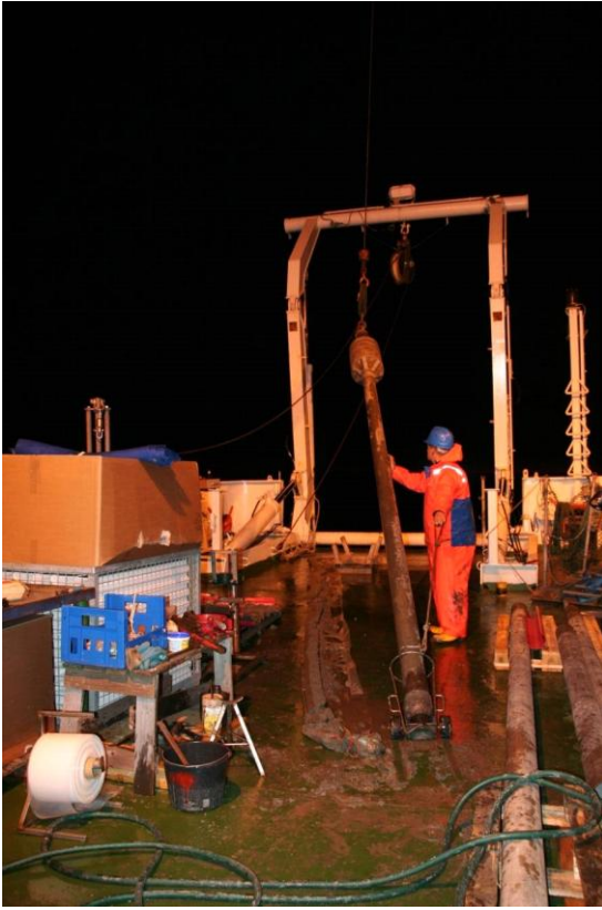
Figure 2. Taking a 6m long gravity core (a) and a multi core (b).
