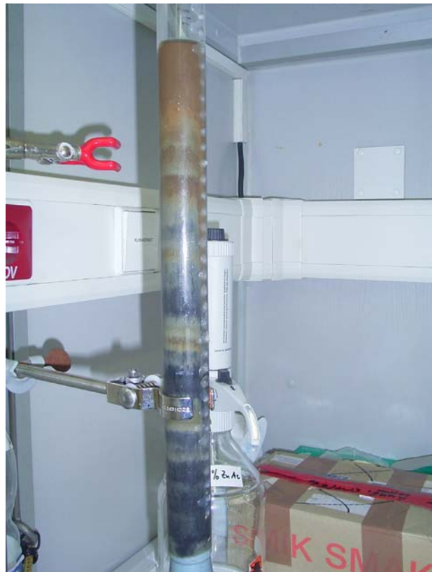
Figure 2. Multicorer from Station 372820 Bothnian Bight
